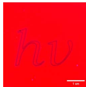
Figure 3. 1a adsorbed on a chromatographic silica gel plate visualized by 366 nm light. The hv symbol was created by a green laser light.
